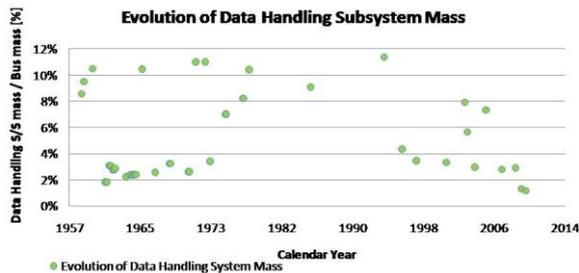
Figure 12: Evolution of data handling subsystem mass of exploration systems from 1958 to 2010
