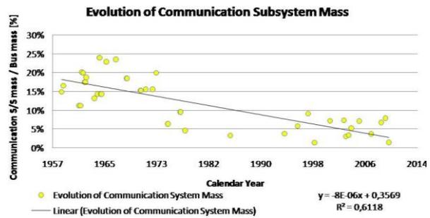
Figure 13: Evolution of communication subsystem mass of exploration systems from 1958 to 2010
