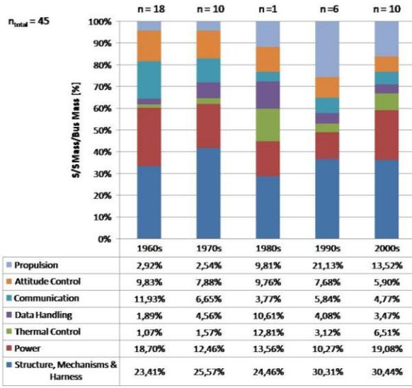
Figure 8: Evolution of relative average subsystem masses grouped by decades from 1960s to 2000s
