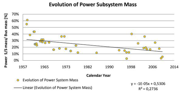
Figure 10: Evolution of power subsystem mass of exploration systems from 1958 to 2010
