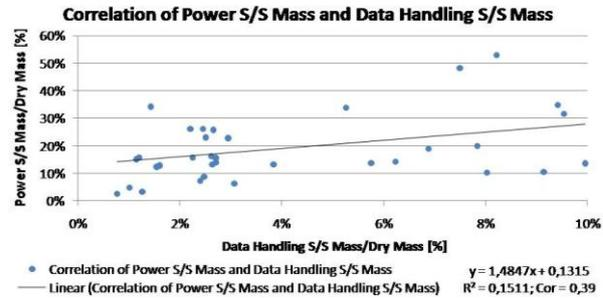
Figure 15: Correlation of power S/S mass and data handling S/S mass of exploration systems (1958 to 2010)
