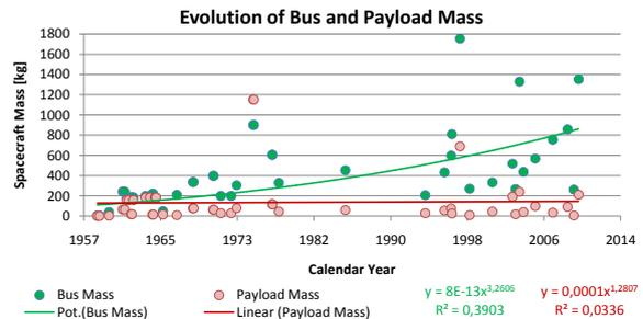
Figure 7: Evolution of bus and payload mass of exploration systems from 1958 to 2011
