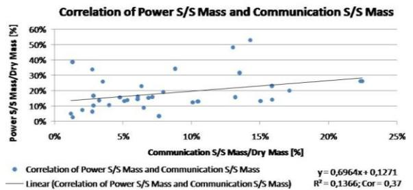
Figure 16: Correlation of power S/S mass and communication S/S mass of exploration systems (1958 to 2010)
