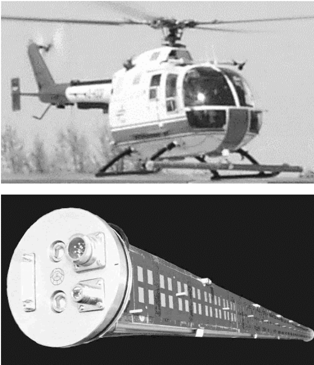
Figure 4: Top: Antenna system attached to the skids of the helicopter. Bottom: RF side of the SIREV antenna with the 56 2\lambda patch receiving subarrays. A detailed description of antenna hardware may be found in [12].
