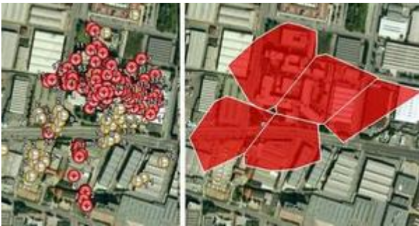
Figure 2. From positions to places : how a set of coordinates (left) is transformed into places (right)
