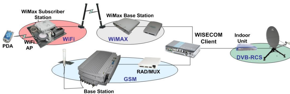
Figure 4: GSM and WiFi/WiMAX over DVB-RCS architecture
