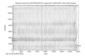
**Figure 5** Residual plot between object points coordinates derived from the direct model and those re-calculated by RPCs for the forward image of the PRISM sensor. At bottom-right the size of one pixel is shown.
