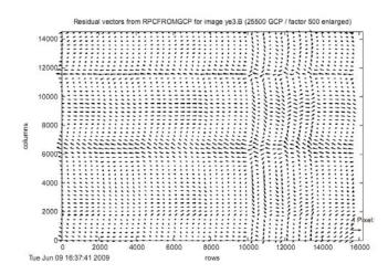
**Figure 4** Residual plot between object points coordinates derived from the direct model and those re-calculated by RPCs for backward image of the PRISM sensor. At bottom-right the size of one pixel is shown.
