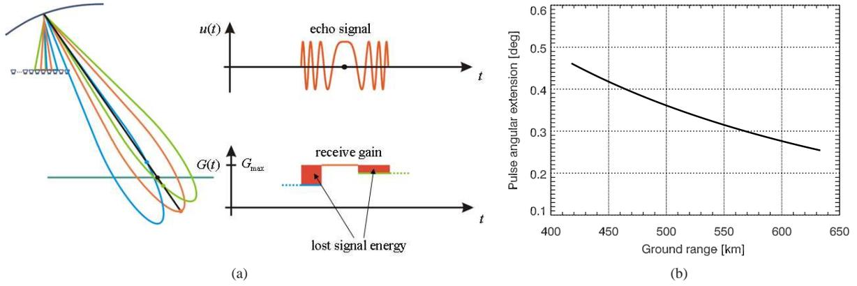
Fig. 2. a) Pulse extension loss principle. b) Angular pulse extension on ground as a function of ground range.
