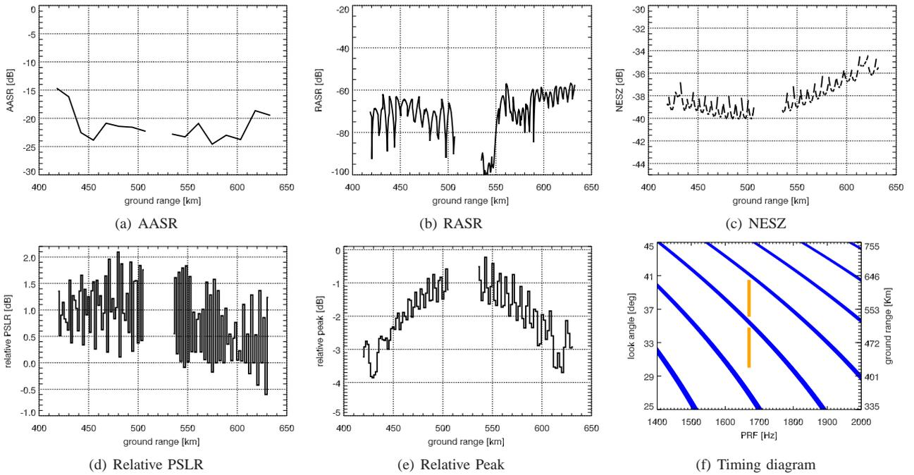
Fig. 4. DBF SAR System Performance and the timing diagram.
