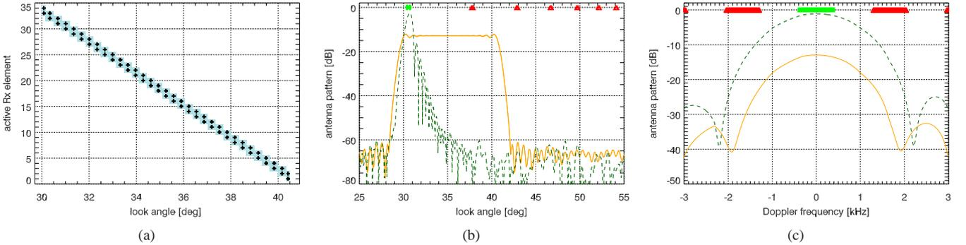
Fig. 3. a) Feed activation matrix as a function of a look angle. b) and c) Elevation and azimuth antenna patterns correspondingly (solid line - Tx, dashed line - Rx).
