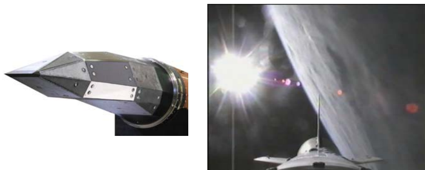
Fig. 1: October 27th, 2005 the SHarp Edge Flight EXperiment-I (SHEFEX-I) performed its successful flight. Left: flight configuration. Right: onboard camera view with Sun and Earth at the back.
