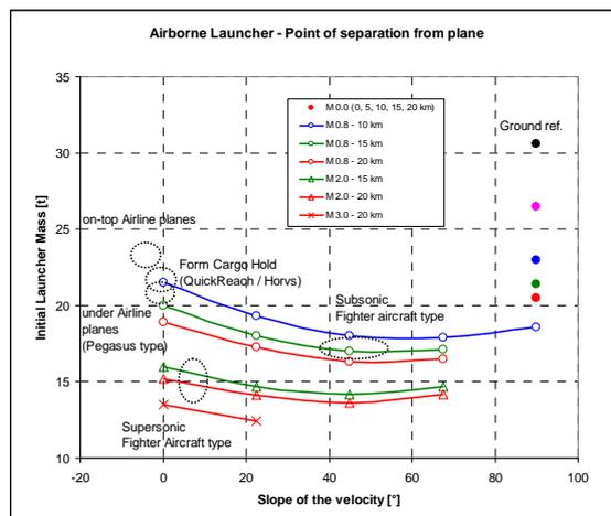
Figure 8: launch vehicle initial mass for lift-off or separation (airborne) conditions versus: altitude, MACH number and path angle.
