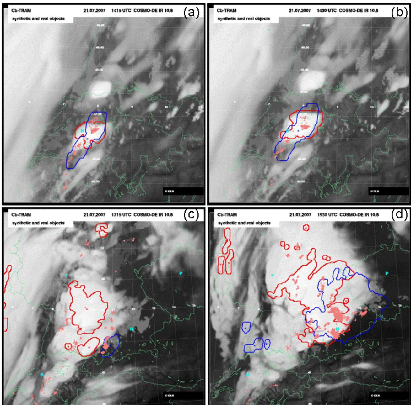
**Fig. 6** Comparison of forecasted synthetic top volumes (red contours) with observed top volumes (blue contours) of mature thunderstorms detected by Cb-TRAM<sub>COSMO</sub> and Cb-TRAM, respectively, over Switzerland at (a) 14:15 UTC and (b) 14:30 UTC and over Germany and the Alpine region at (c) 17:15 UTC and (d) 19:30 UTC on 21 July 2007. The background is the IR 10.8  $\mu\text{m}$  synthetic satellite image forecasted by the 00 UTC COSMO-DE model run.
