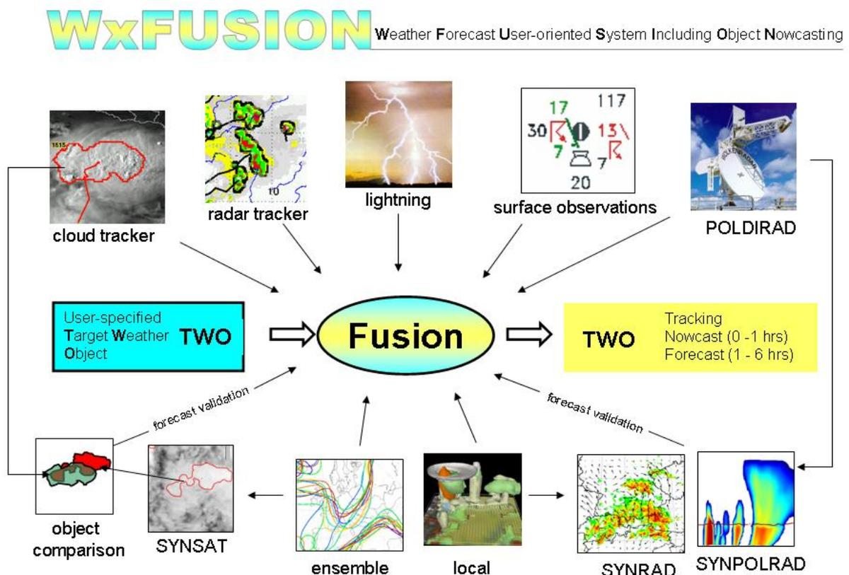
**Fig. 1.** Schematic diagram of the WxFUSION concept. User specified target weather objects (TWO) are characterized by appropriate information through a fusion of selected nowcast information (upper half) and forecast products (lower half).
