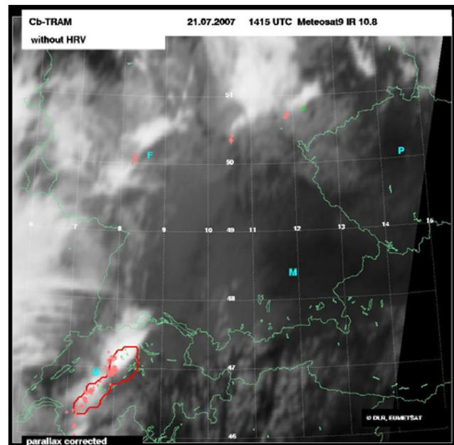
**Fig. 4** Thunderstorm top volumes detected by Cb-TRAM (red contours) and LINET lightning data (pink crosses) superimposed on the IR 10,8  $\mu\text{m}$  METEOSAT image over Germany and the Alpine region on 21 July 2007 at 14:15 UTC. Bern, Frankfurt, Munich Airport, and Prague are marked by the turquoise letters B, F, M, and P, respectively.
