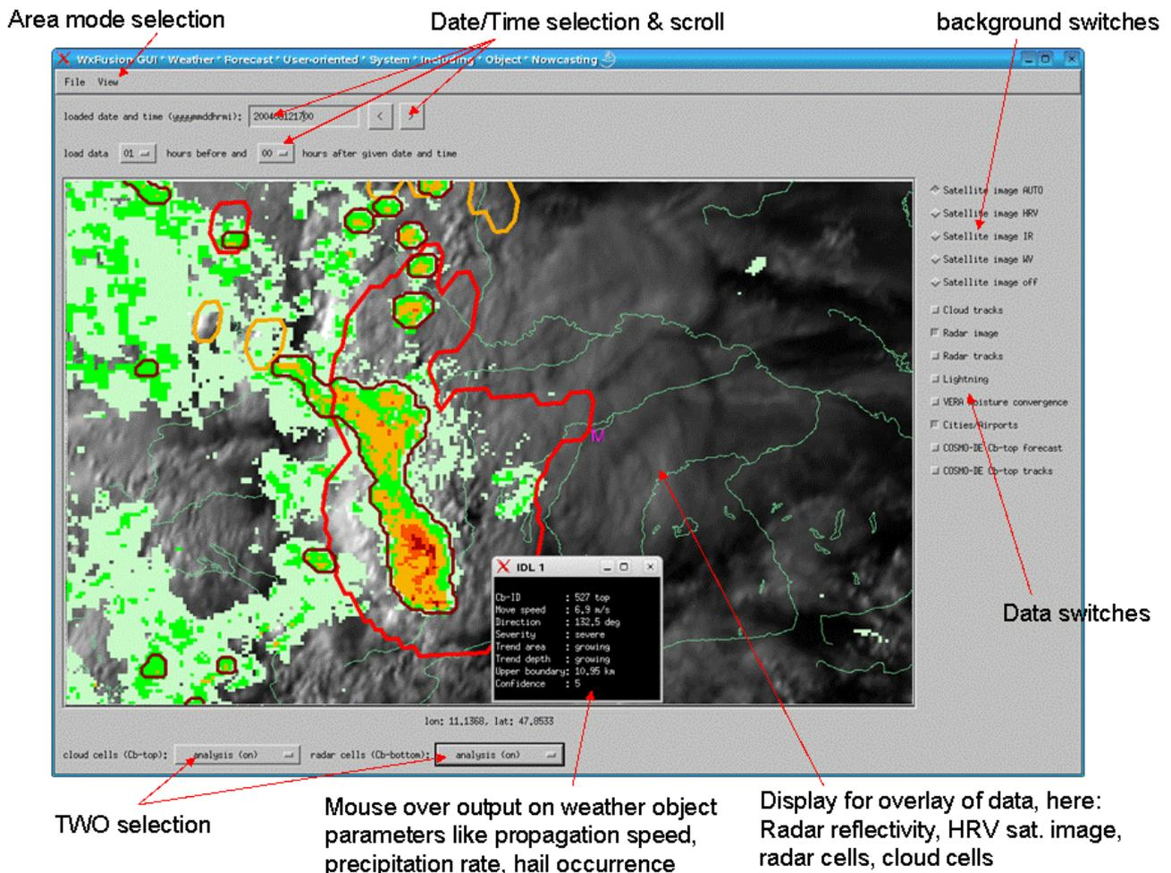
**Fig. 3** WxFUSION graphical user interface displaying radar reflectivity (colored shading), radar cells with reflectivity  $\geq 37$  dBZ (dark red contours) and cloud cells (orange and red contours) superimposed on the HRV satellite image (grey and shading) for the TMA Munich on 12 August 2004 at 17:00 UTC. Munich airport is marked by a purple M. Rivers and the contours of lakes are indicated in green.
