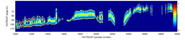
**Figure 4:** E-SAR L-band (HH-VV) polarization dual baseline (5 m and 10 m) vertical coherence tomography. In all above tomograms initial value of the tree height is derived from HUTSCAT measurement and all tomograms are presented in HUTSCAT coordinates. The ground phase is derived from RVoG model inversion for L-band. The x-axis and y-axis as in Fig.1.
