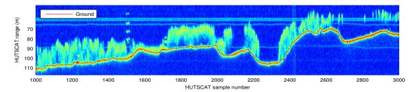
**Figure 1:** The forest vertical scattering profile at X-band, measured by HUTSCAT scatterometer. The ground line is indicated by a red line. Light areas are forest canopy. The x-axis is HUTSCAT sample number, corresponding to helicopter movement. One sample corresponds approximately to 1.25 m. The y-axis is HUTSCAT vertical range in meters. The length of track in the image is about 2.5 km. Flight direction is from right to left.
