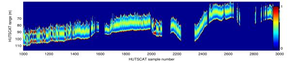
**Figure 5:** E-SAR L-band (HH-VV) polarization dual baseline (5 m and 10 m) vertical coherence tomography. The initial value of the tree height and ground phase is derived from RVoG model inversion. The tomogram is presented in HUTSCAT coordinates. The x-axis and y-axis as in Fig.1.
