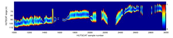
**Figure 3:** E-SAR L-band (HH-VV) polarization single baseline (10 m) vertical coherence tomography. The x-axis and y-axis as in Fig.1.
