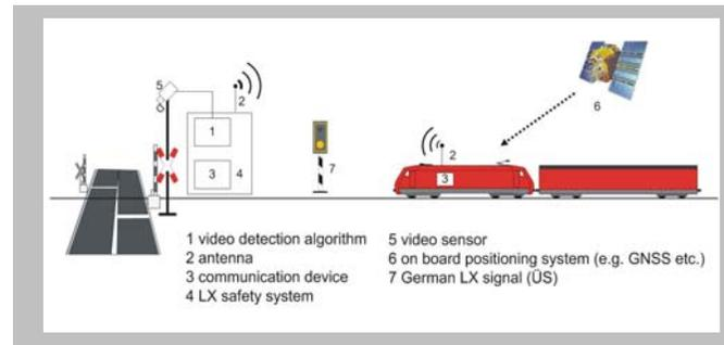
Fig. 3: Layout of the customize technique at AHB
