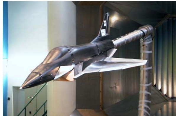
Figure 4: X-31-Remote-Control-Model in the DNW-NWB Braunschweig.
