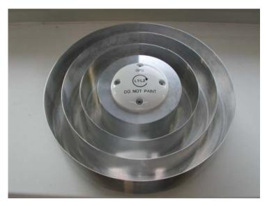
**Fig. 9** GPS antenna and choke ring for the TSX/TDX satellites (engineering model).
