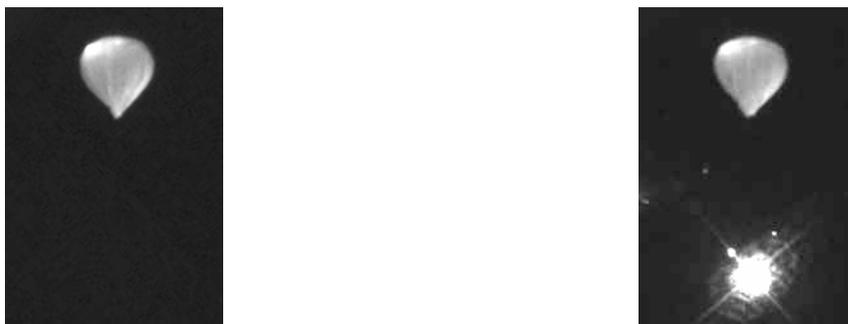
Fig. 15. Near infrared picture from the ground station tracking camera of the stratospheric balloon. Before (left) and after (right) acquisition. The altitude is 23 km and the distance to the ground station approximately 60km
