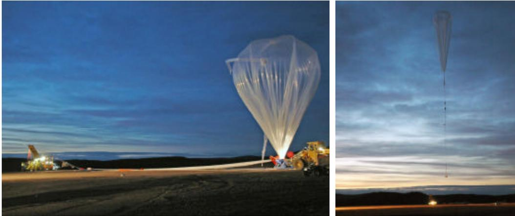
Fig. 11. Picture of balloon before launch with payload at the launch vehicle in the background (left) and flight train at launch (right). The nacelle is located at the bottom of the flight train.
