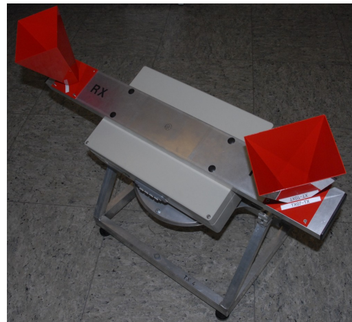
Fig. 6. Active target (transponder). The transponder housing including the antennas can be rotated which results in different scattering matrices.
