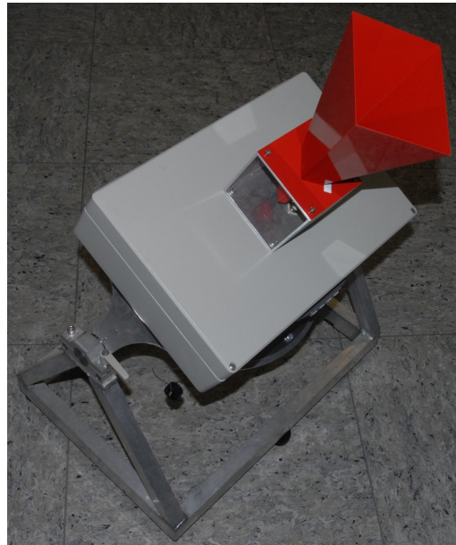
Fig. 3. Ground receiver. The housing can be rotated in steps of 45^\circ to allow polarimetric characterization of the satellite.
