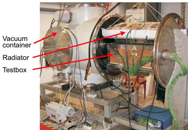
**Fig. 16** Thermal radiation investigation chamber
