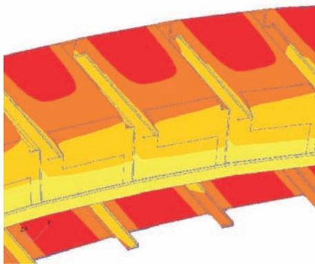
**Fig. 12** Fuselage temperature profile across one frame
