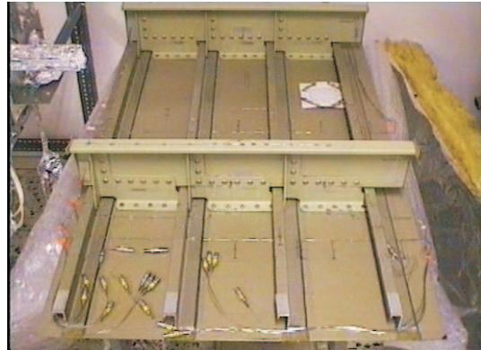
Fig. 9 Glare test panel with stringers and frames
