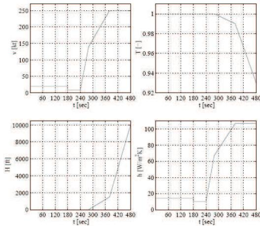
**Fig. 11** Take-off profiles of velocity  $v$ , Temperature  $T$ , Altitude  $H$  and Convection  $h$
