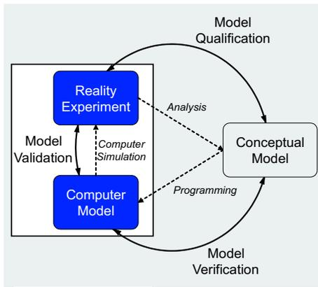
Fig. 2 Simulation tools validation procedure
