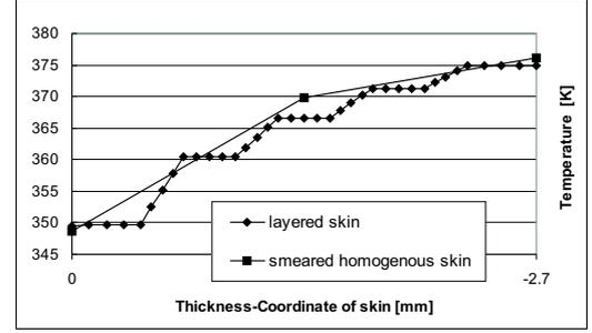
**Fig. 6** Transversal temperature profile for different discretization levels
