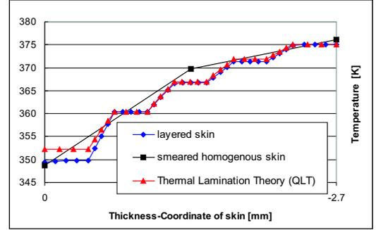
Fig. 14 Comparison of fully 3D and homogenized simulation with thermal lamination theory
