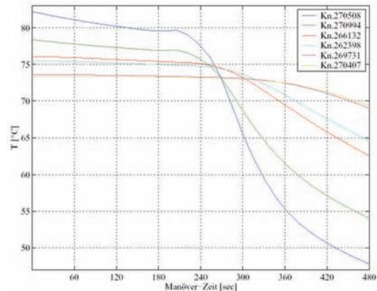
**Fig. 13** Temperature distribution in take-off environment
