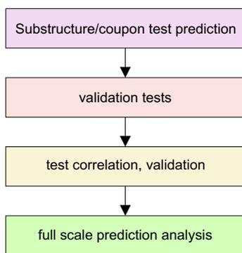
Fig. 3 Virtual testing process flow-chart
