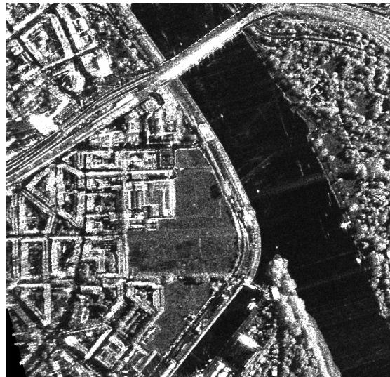
Figure 4. GTC with adjustment to laser-scanning DEM
