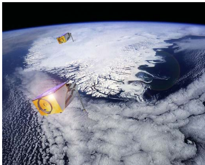
Fig. 1: Artist's impression of two ICEDANCE SAR satellites flying in close formation ( DEM mode ), precisely measuring surface elevation of cryospheric key regions of the greenlandic ice sheet.
