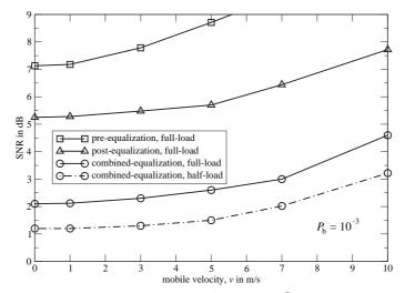
*Figure 7.* SNR required to achieve a BER of  $P_{\rm b} = 10^{-3}$  versus mobile speed v for uplink MC-CDMA with combined-equalization, post-equalization, or pre-equalization.
