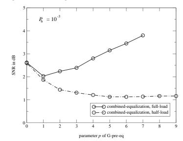
Figure 4. SNR required to achieve an average BER of  $P_{\rm b} = 10^{-3}$  versus the G-preeq parameter p for adaptive uplink MC-CDMA with combined-equalization.
