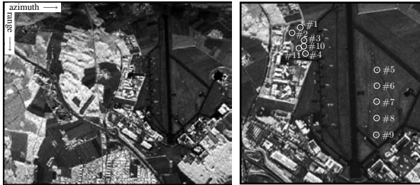
Figure 1: (left) Reflectivity image of the scene under study and (right) detail of corner reflectors.
