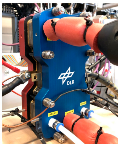
Figure 4. Fuel cell stack of DLR installed on the test bench.
