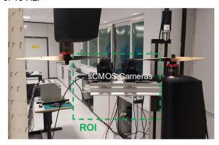
Figure 3 PIV set-up for tandem case in CIRA
