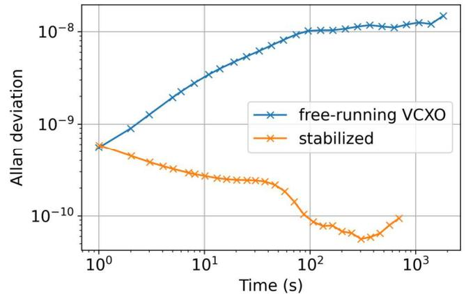
Fig. 2. Allan deviation (of the normalized data) of stabilized measurements with CO as well as of the free-running TX VCXO.
