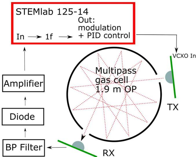
Fig. 1. Scheme of the absorption spectroscopy setup including the control loop for the stabilization of the TX frequency.
