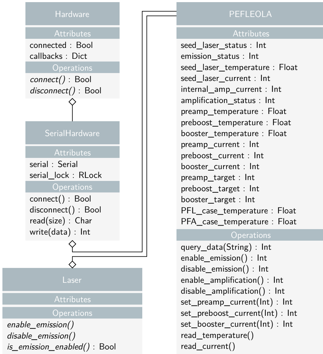
Figure 3.6: Unified Modeling Language (UML) diagram of the laser control backend: the Hardware super class implements the general attributes and methods of an abstract hardware controller. The SerialHardware parent class inherits from Hardware and implements serial communication methods. The Laser class defines methods for the overall control of multiple laser sources [26]. The PEFLEOLA class implements the Laser parent class stub methods and additional surveillance methods to interact with the PFL, PFA and the Hyperion GUI. Some methods have been omitted for clarity.
