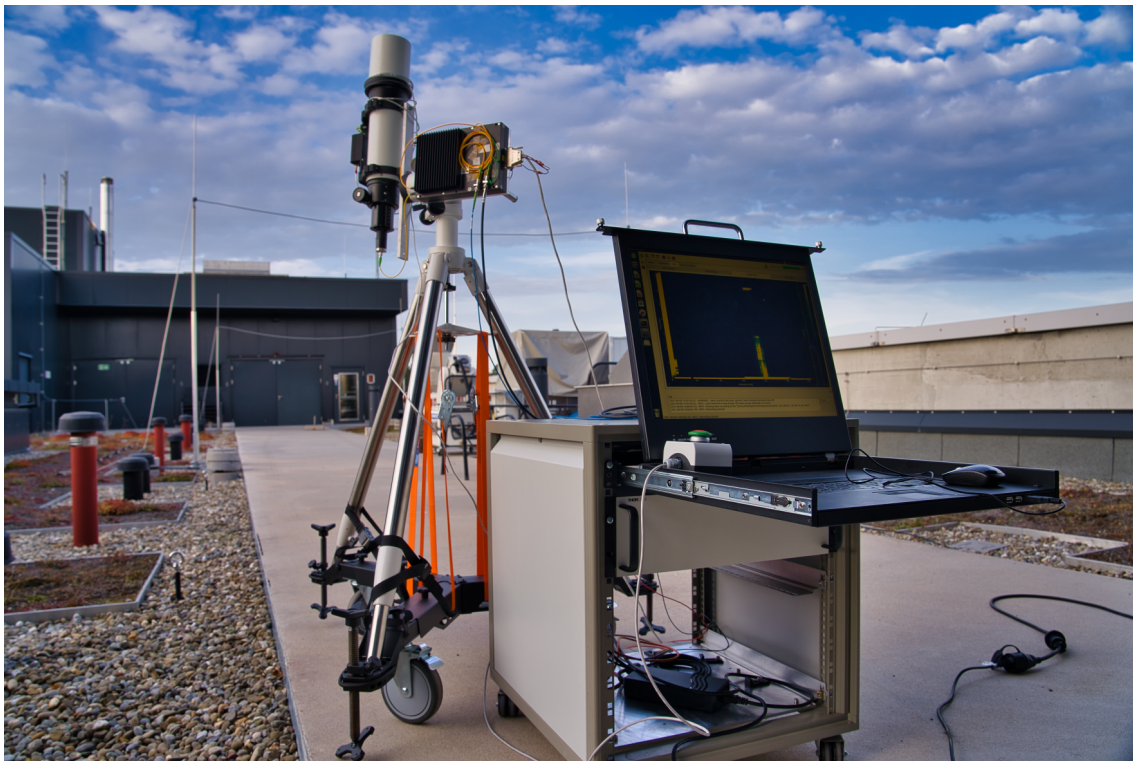
Figure 7.1: Active lidar system at the DLR site in Stuttgart-Vaihingen. This image was taken during the September 25th, 2021 field campaign intended to measure volcanic aerosols. The rack in the foreground contains the evaluation electronics and parts of the optical system. The monostatic setup as well as the pulsed fiber amplifier are mounted on the stand. A live feed of the lidar spectrum updating at about 1.2 Hz can be seen on the integrated monitor.
