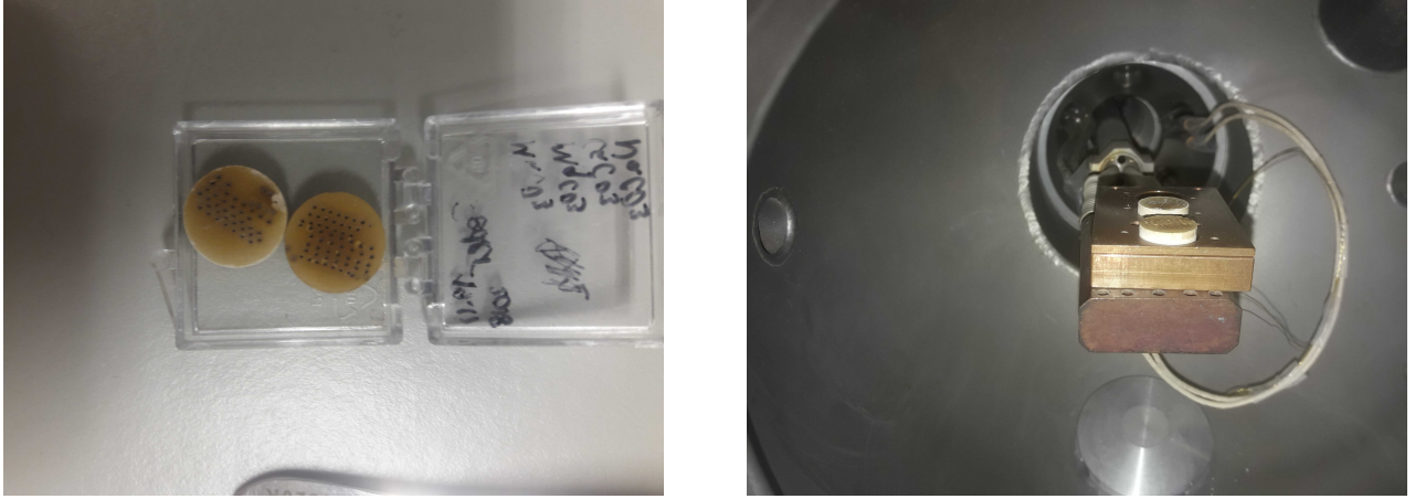
Figure 3.2.1: left: A photo of two pellets from mixed carbonates. Small craters from LIBS measurements can be seen on the surface of the pellets. right: The pellets located in the simulation chamber wherein the measurements have been performed.
