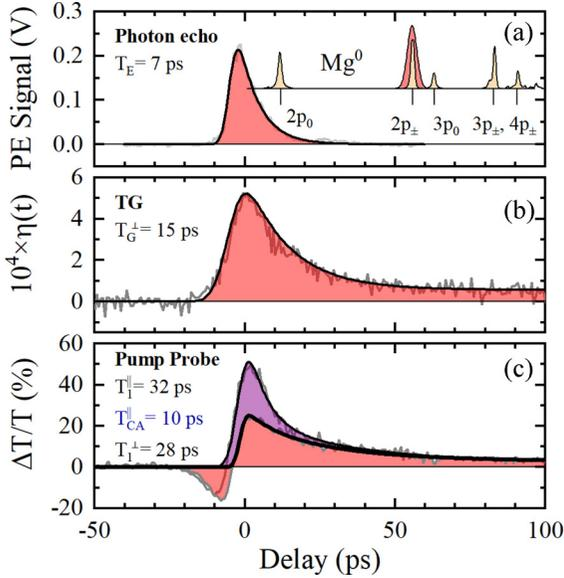
FIG. 6. Comparison of photon echo (a), transient grating (b), and PP (c) signals measured with FELIX when pumping resonantly (see inset) for the  $\text{Mg}^0 1s(A_1) \rightarrow 2p_{\pm}$  transition (Si:Mg sample 138-2). The coherent artifact (CA) appears in the PP signal [(c), purple] when the pump and probe beams are parallel polarized. The FEL pump spectrum (red) and Si:Mg absorption spectrum (light brown) are shown in scale.
