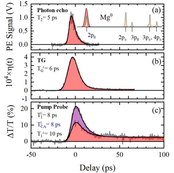
FIG. 5. Comparison of photon echo (a), transient grating (b), and pump-probe (c) signals measured with FELIX when pumping resonantly (see inset) for the  $\text{Mg}^0 1s(A_1) \rightarrow 2p_0$  transition (Si:Mg sample 138-2). The coherent artifact (CA) appears in the PP signal [(c), purple] when the pump and probe beams are parallel polarized. The FEL pump spectrum (red) and Si:Mg absorption spectrum (light brown) are shown in scale.
