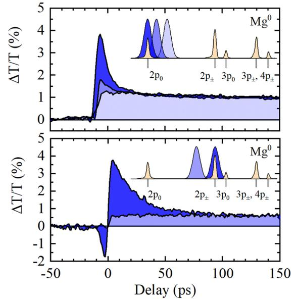
FIG. 3. Pump-probe signals for the  $\text{Mg}^0 1s(A_1) \rightarrow 2p_0$  (top) and  $2p_\pm$  (bottom) transitions (Si:Mg sample 98-1) in and out of resonance measured with FELBE. The signals consist of two components recovering on different timescales. The short component vanishes when tuning the FEL out of resonance. The FEL pump spectrum (blue) and Si:Mg absorption spectrum (light brown) are shown in scale.
