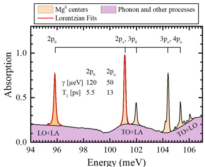
FIG. 1. FTIR absorption spectrum of a Si:Mg sample (sample 138-2) at  $\approx 15 \text{ K}$ . For better distinction the resonant absorption lines are separated from the two-phonon background spectrum (purple) obtained for an undoped Si reference sample. The  $2p_0$  and  $2p_{\pm}$  lines are fitted with (saturated) Lorentz functions. LA, longitudinal acoustic; LO, longitudinal optical; TO, transverse optical.
