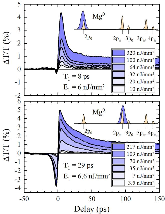
FIG. 4. Intensity-dependent pump-probe signals for the  $\text{Mg}^0 1s(A_1) \rightarrow 2p_0$  (top) and  $2p_{\pm}$  (bottom) (Si:Mg sample 98-1) transitions on resonance (see insets) measured with FELBE. The decay time of the short component remains unchanged with changing the laser intensity for both transitions. The FEL pump spectrum (blue) and Si:Mg absorption spectrum (light brown) are shown in scale.
