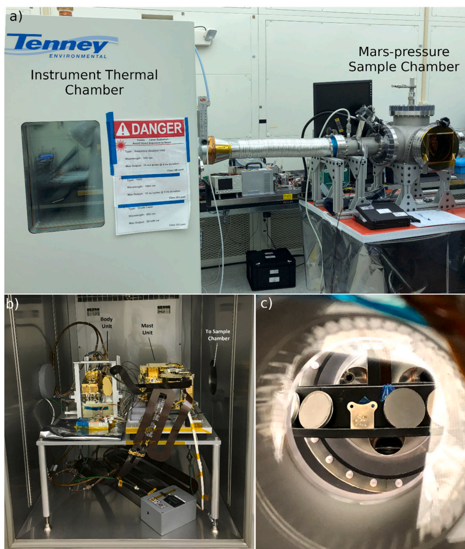
Fig. 1. Photographs of the laboratory setup: (a) environmental chamber, with a tube connecting to the chamber containing standards to be analyzed; (b) SuperCam inside the environmental chamber and (c) view down the connecting tube of several pressed powder samples and a Ti plate ready for analysis. Photo credit: R. Wiens.
