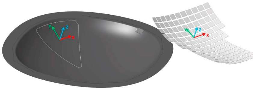
Fig. 6. Axis alignment at the end-effector TCP and the on the tooling surface
