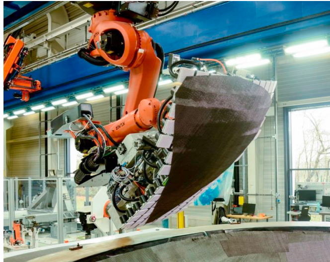
Fig. 2. The Modular Gripper with textile after deformation
