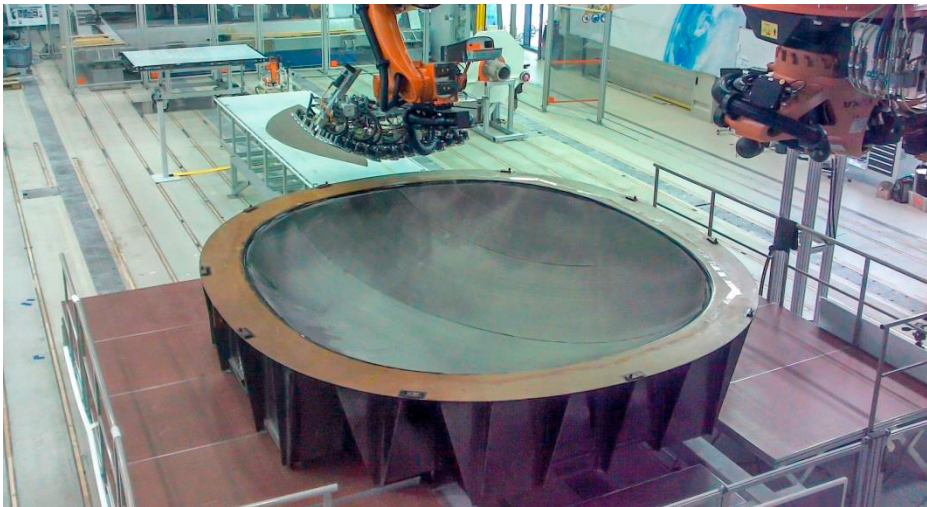
Fig. 1. Rear Pressure Bulk Head tooling in the robot cell
