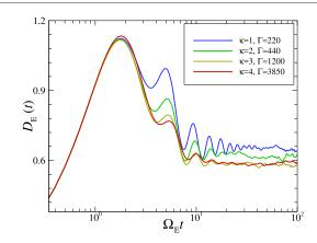
Figure 3. Time-dependent reduced self-diffusion coefficient  $D_{\rm E}(t)$  versus the reduced time  $t\Omega_{\rm E}$  for Yukawa melts characterized by four different  $\kappa$ -values. The color notation is the same as in figure 2. The diffusion coefficient is determined from the Green-Kubo relation (i.e. using VAF) and is normalized as  $D_{\rm E} = D(\Omega_{\rm E}/v_T^2)$ .
