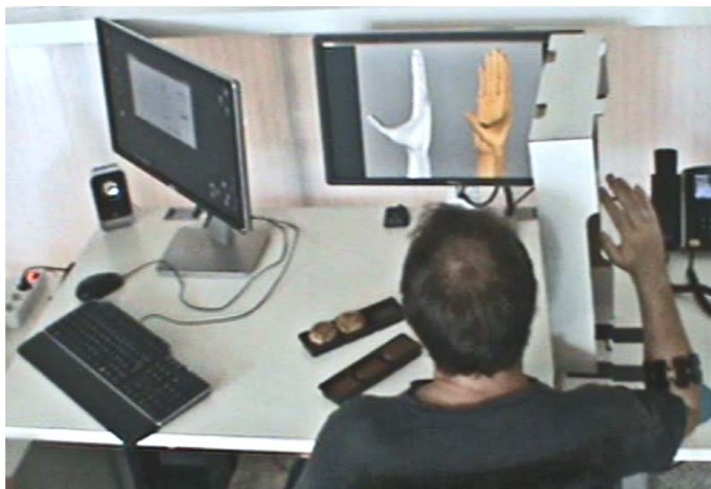
Figure 2 • The experimental setup while a subject performs Experiment 0, MT. The stimulus (white hand) and the “prosthesis” (skin-textured hand) are displayed on the screen; the subject’s right arm (wearing the Myo bracelet) and hand are shielded from view using a cardboard partition.
