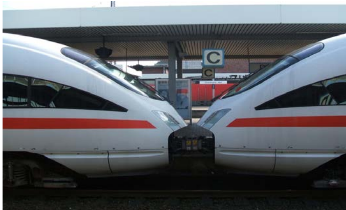
Figure 3: ICE3 with mechanical connection at a station, (www.bahnbilder.de,2018)
