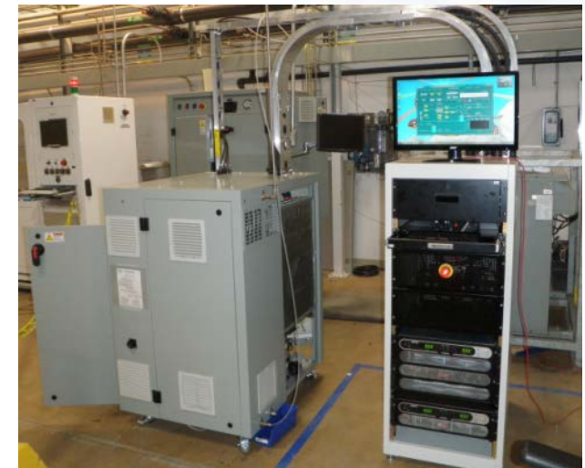
0.75 - 2.5 Nm 3 H 2 h -1 “Hylyzer” PEM electrolyzer unit, 8 bar
