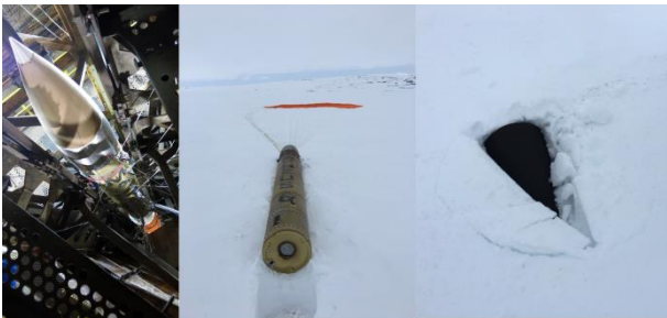
Figure 10. MAPHEUS 6 in the Skylark tower (left), payload (mid) and cork coated FNC recovery (right).
