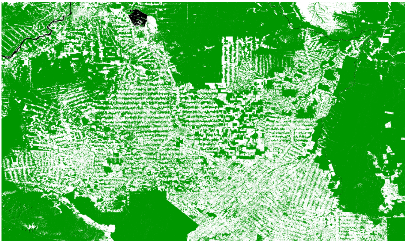
Fig. 3. Forest map of an area in Rondonia/Brazil derived from TanDEM-X coherence quick looks (50 m x 50 m resolution).
