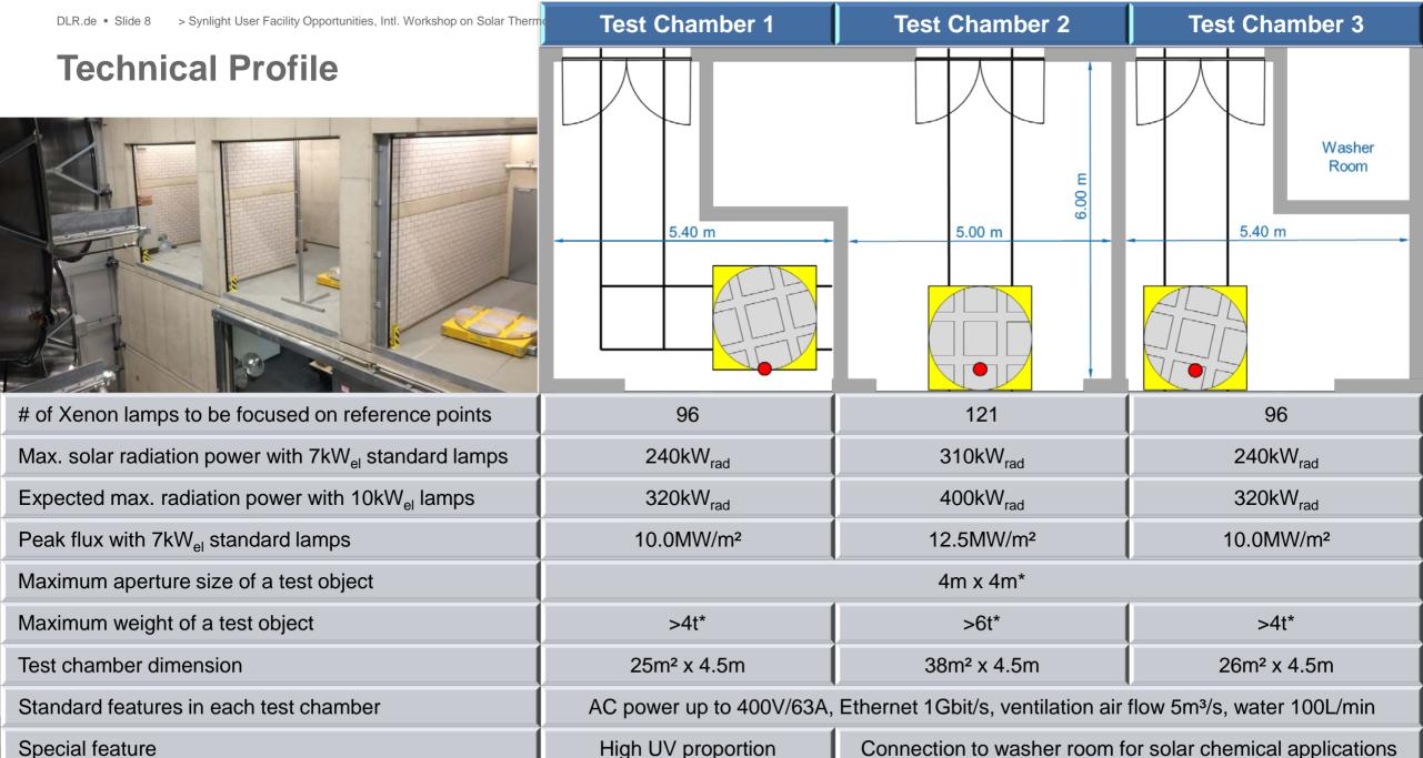
\* Test objects up to 2.5t and 2m x 2m x 2m can be transported and positioned on manually moveable trolleys
