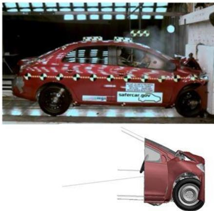
**Fig. 23: Comparison of crash behaviour obtained in the full vehicle crash test and in the simulation using the simplified vehicle model (crash test image Toyota Yaris from [28])**
