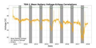
**Figure 5**: Mean and minimum TDX-1 battery voltage over mission duration with eclipse
