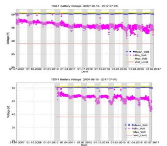
**Figure 1**: Battery voltage per day over mission duration and eclipse periods. Upper plot: TSX-1, lower plot: TDX-1
