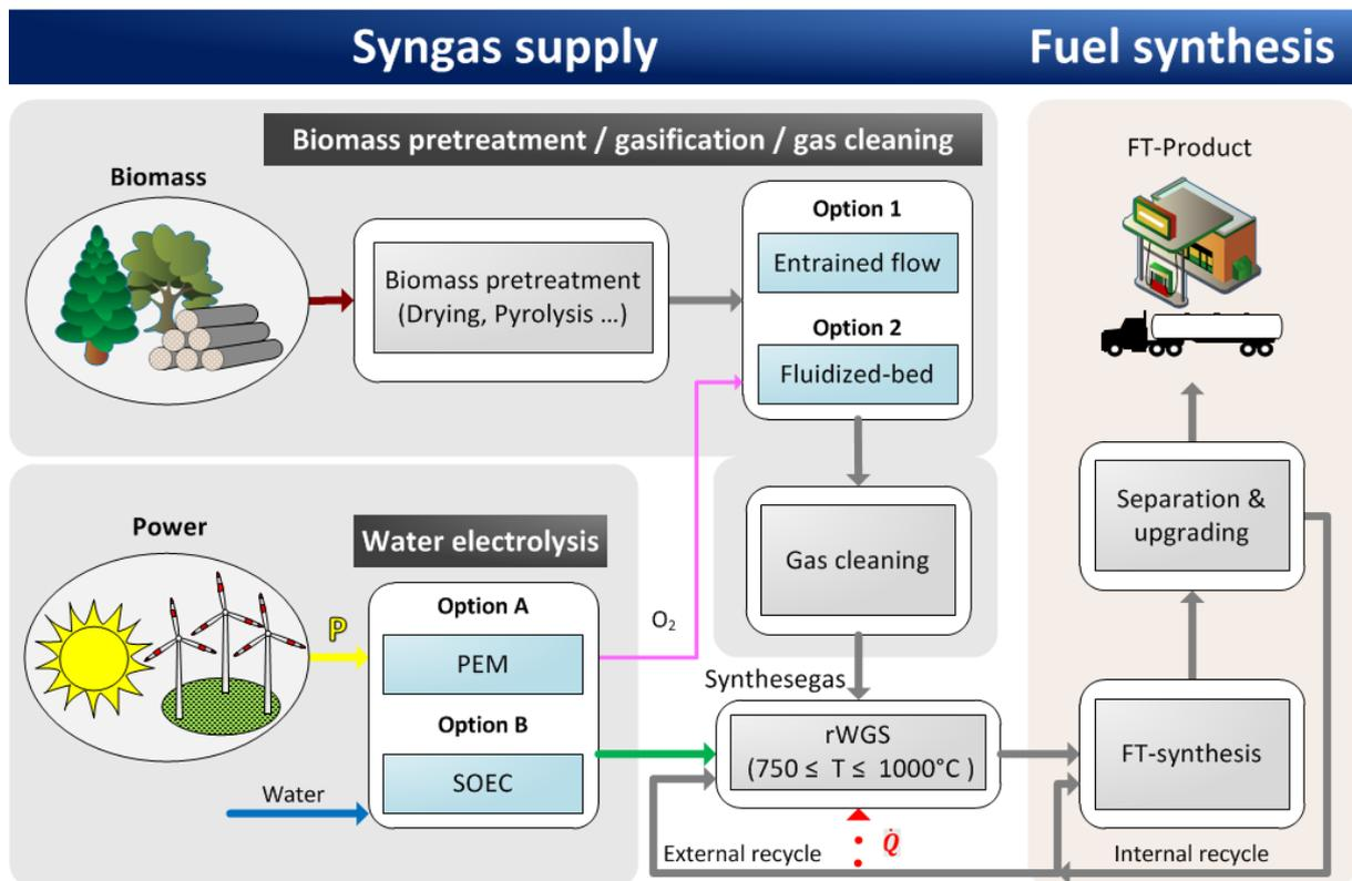
Figure 1: Block flow diagram and system boundary of PBtL concept
