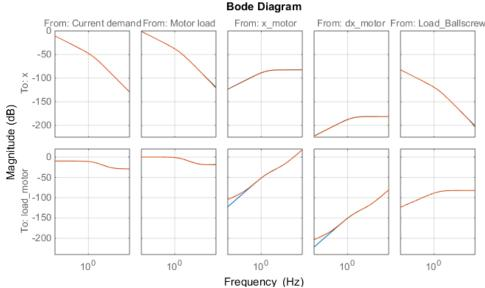
Figure 2. Excerpt of the bode plots of the system (red) and the reduced system (blue)
