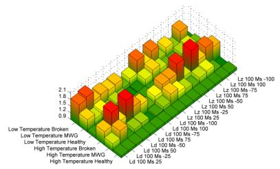
Figure 5. Detectability of the gear faults using only available sensors on the actuator. A higher number indicates a better detectability. The loading condition marked with Ld stand for a compressive load, Lz for tension loads on the actuator. The measurements marked with MWG are the results of the measurements with a plastic deformation of one tooth. Low temperature denotes room temperature and high temperature an elevated temperature  $(+70^{\circ}C)$ .
