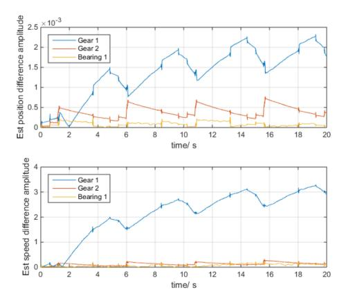
Figure 4. Simulation results of a harmonic analysis of a gear with a fault on the first stage.
