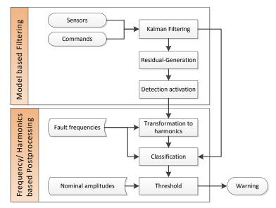
Figure 1. Structure model- and harmonics based health monitoring.
