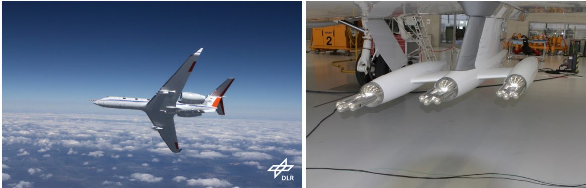
Figure 11. DLR HALO aircraft with particle measurement system (PMS carrier) installed under the wing
