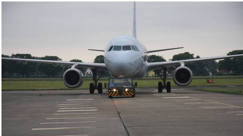
Figure 6. Taxi Vibration Test on the DLR research aircraft ATRA, an A320-200
