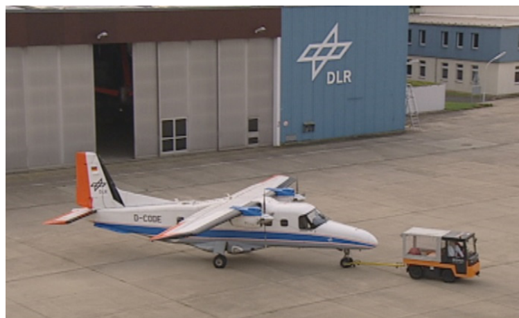
Figure 3. Taxi vibration test on Do228 commuter class aircraft pulled by a tractor in front of the old DLR flight operations hangar in Braunschweig, Germany
