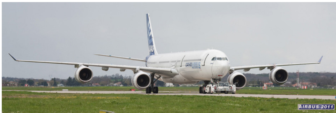
Figure 8. Taxi Vibration Test on an A340-600 long range aircraft at Airbus in Toulouse
