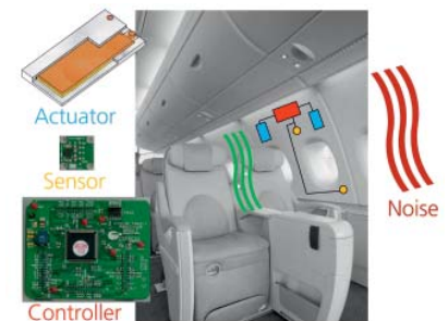
Fig. 1: Principle of Smart Lining Technologie.
