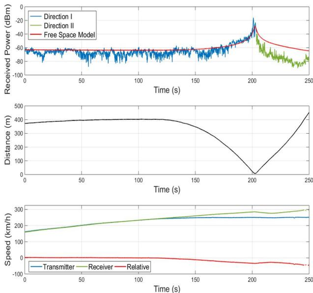
Fig. 5: High speed overtaking maneuver in rural environment.
