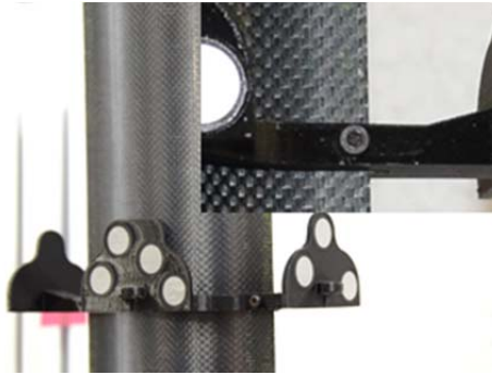
b) Visual/Load adapter for later bending
