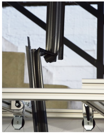
b) Column buckling and destruction under axial compression
