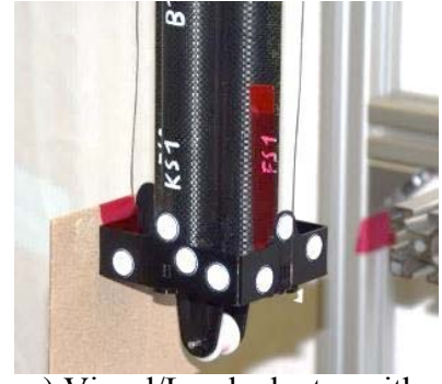
c) Visual/Load adapter with pulley for axial compression loading
