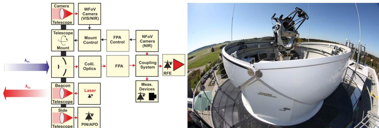
**Fig 5.** Left: generic functional block diagram of OGS-OP; Right: Image of open dome with 40 cm Cassegrain telescope (Image Source: DLR).
