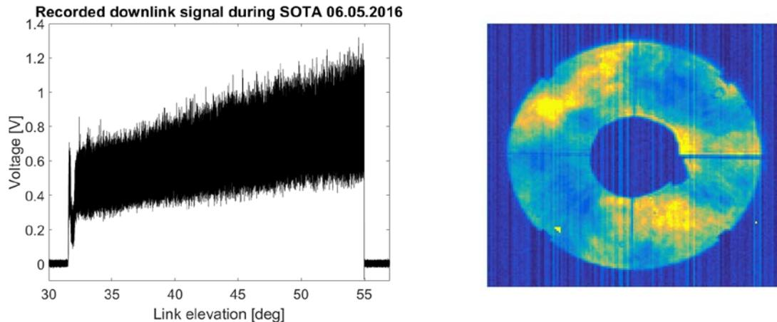
**Fig 8.** Left: recorded scintillation signal during SOTA downlink. Right: example of unprocessed pupil camera image of scintillation signal. (Image source: DLR)
