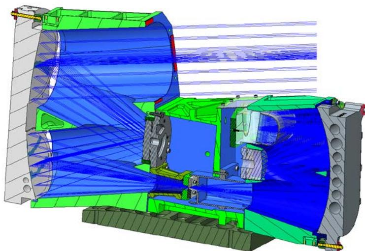
**Fig. 8.** Cut-view of the opto-mechanical system. The TMA is on the left side, the spectrometer on the right one.
