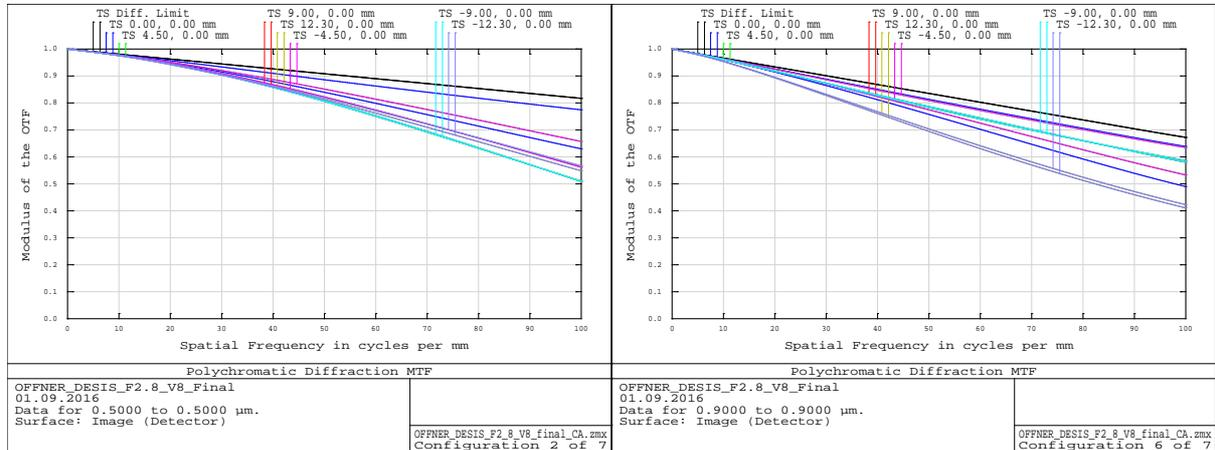
**Fig. 7.** Modulation transfer function (MTF) of the spectrometer for wavelengths of 500 nm (left), and 900 nm (right), respectively.
