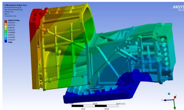
Fig. 12. Deformation (mm) of the system under gravity load in Y-direction (vertical).
