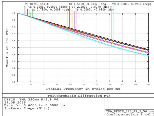
Fig. 2. Modulation transfer function (MTF) of the TMA.
