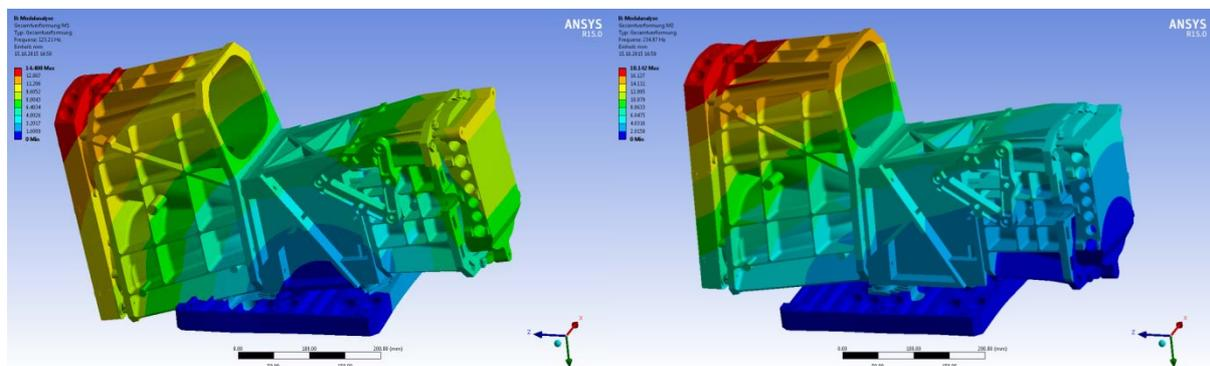
Fig. 11. Vibrational Eigenmodes of the opto-mechanical system. The fundamental mode at 123 Hz is shown in the left, while the second mode at 235 Hz is shown in the right picture.
