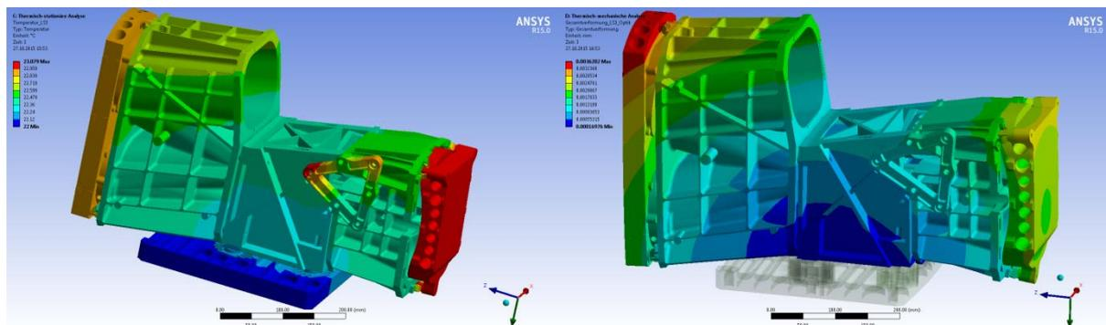
Fig. 13. Temperature distribution (K, left) and deformation pattern (mm, right) due to a thermal flux of 10 W/m<sup>2</sup> onto the top side of the instrument.
