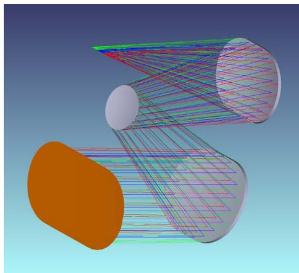
Fig. 1. Lay-out of the TMA.
