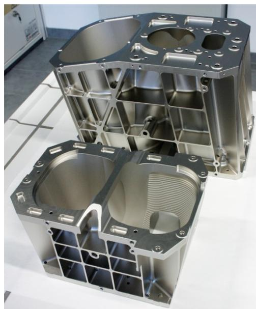
**Fig. 10.** TMA (top) and spectrometer (bottom) housing elements prior to coating.
