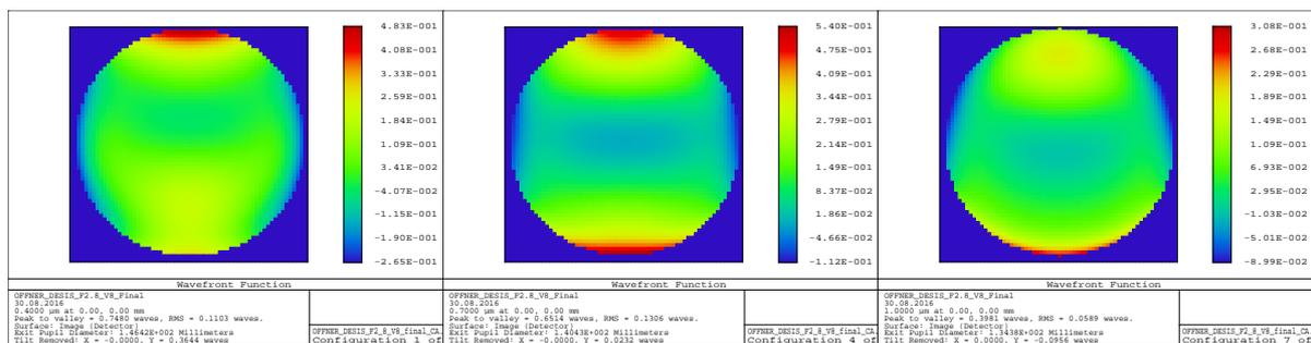
**Fig. 6.** Wavefront errors of an Offner spectrometer with a freeform mirror. Values are given for 400 nm, 700 nm, and 1  $\mu\text{m}$ , respectively.
