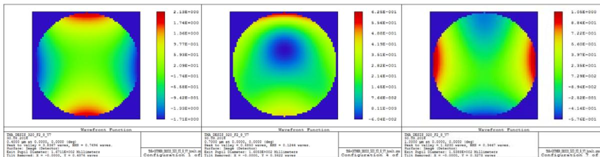
Fig. 4. Wavefront errors of an Offner spectrometer with spherical mirrors. Values are given for 400 nm, 700 nm, and 1  $\mu\text{m}$ , respectively.
