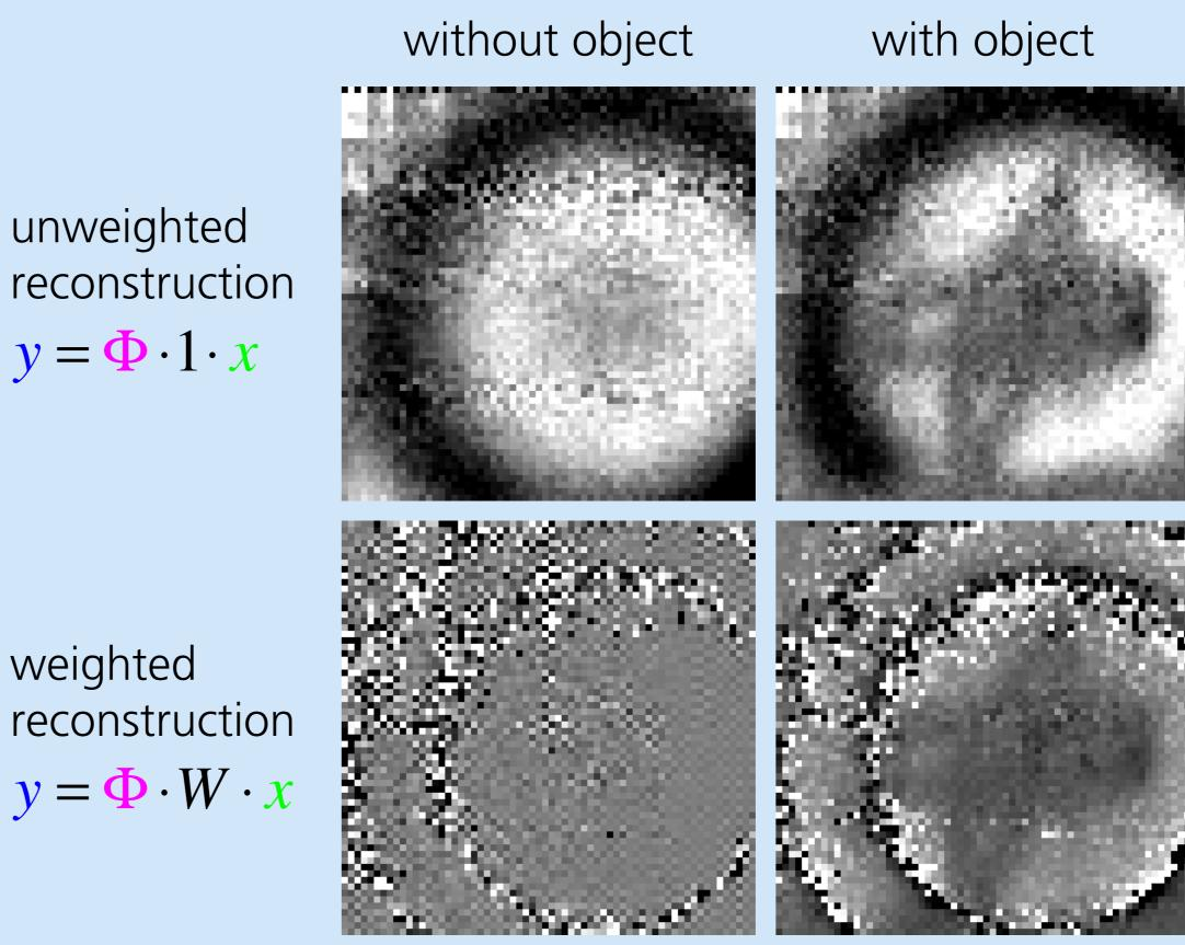
Periodic ring structure around the imaged scene, limiting the field of view of the THz single pixel camera
