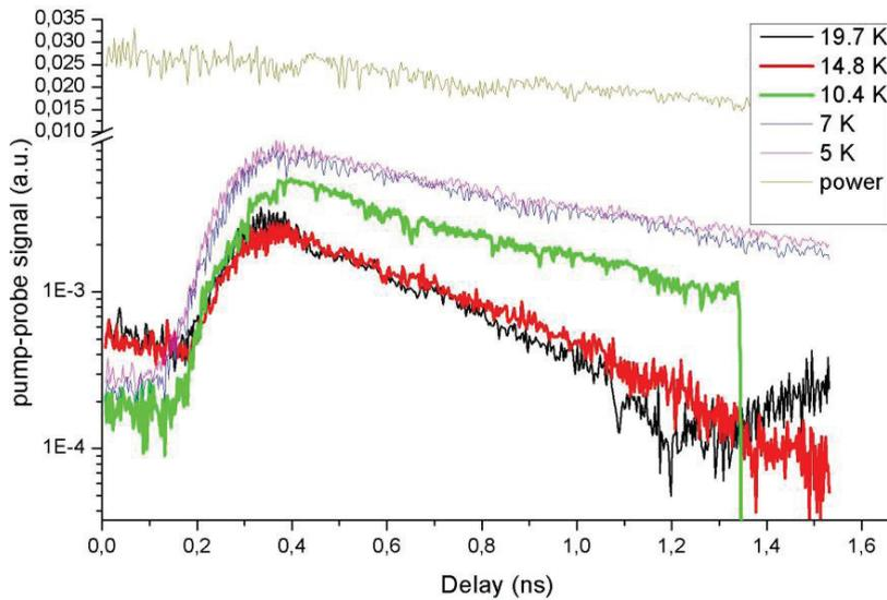
Fig. 4. Pump probe signals vs. delay time for the Ge:Sb sample at 141  $\mu\text{m}$  wavelength at different sample temperatures; the upper signal demonstrates variation of input power during one of the experiments.
