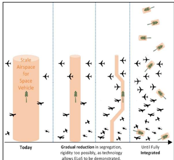
**Figure 4: Dynamic Flight Corridor Handling**
