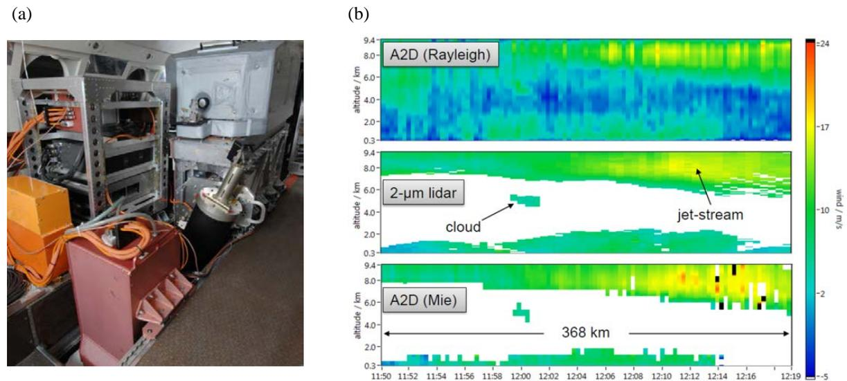
**Fig. 3.** (a): The ALADIN airborne demonstrator (A2D), in the background, mounted together with the 2- $\mu$ m wind lidar onboard the Falcon. (b): Wind measurements from a 367 km long flight track along the East coast of Greenland with the 2- $\mu$ m wind lidar (middle), the A2D Rayleigh (top) and Mie channel (bottom) on 26 September 2009.
