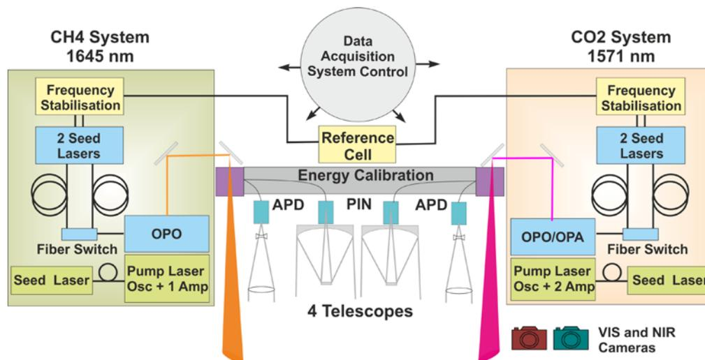
**Fig. 6.** Schematic set-up of the airborne CO<sub>2</sub> and CH<sub>4</sub> integrated path differential absorption lidar.
