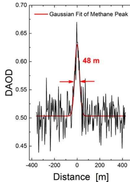
**Fig. 7.** CHARM-F, the combined CO<sub>2</sub> and CH<sub>4</sub> IPDA installed on-board the HALO research aircraft (a) and a narrow methane plume detected as an enhancement of the differential absorption optical depth (DAOD) along the flight path (b).
