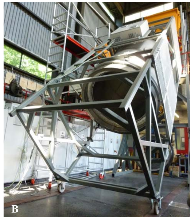
FIGURE 5: SET-UP OF THE CENTREC SCALED UP PROTOTYPE (A) SCHEMATIC DESIGN; (B) PHOTOGRAPH (WITHOUT COLLECTION RING)
